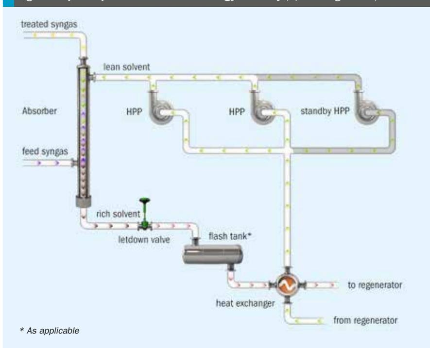
Fig 4: Simplified process flow with energy recovery (3/2 configuration)
