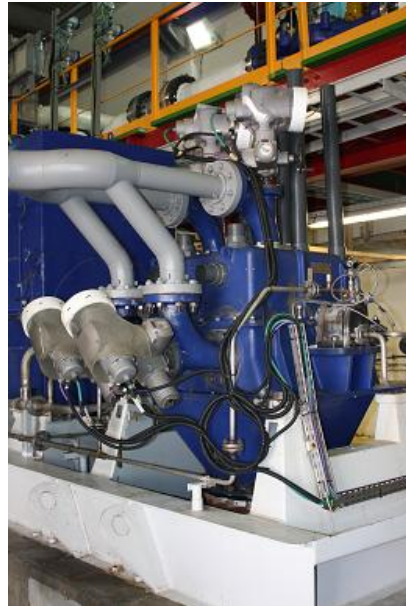
Figure 2 – Palmachim Two-Runner ERT
