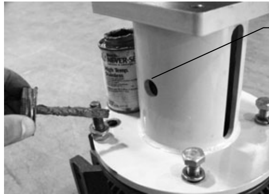
Figure 7-29 - Install Coupling and Bell Housing
