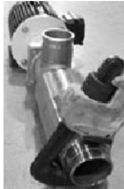
Figure 7-44 – Tighten Outlet Nozzle
