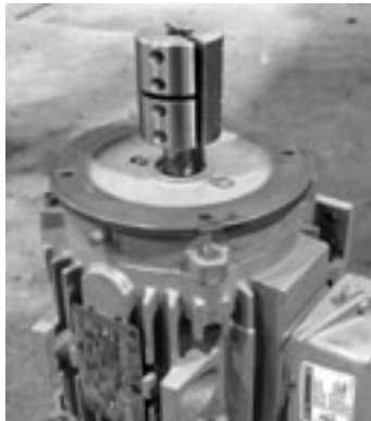
Figure 7-29 - Install Coupling and Bell Housing
