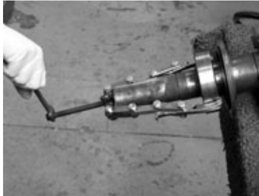
Figure 7-49 – Pull Bearing with Bearing Puller
