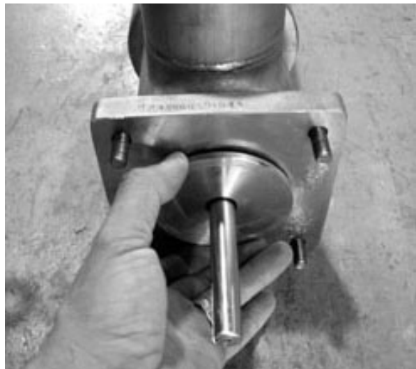
Figure 7-5 - Remove Seal Plate from Inlet
