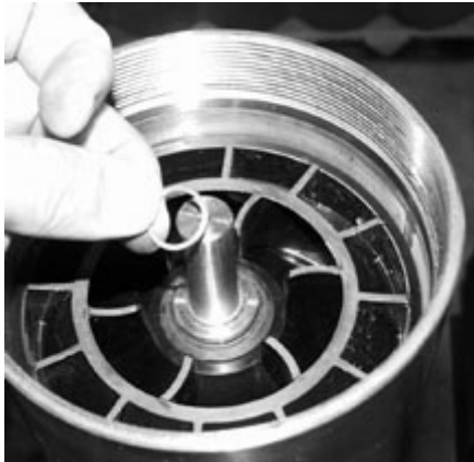
Figure 7-40 - Install Snap Ring, 2400-Series
