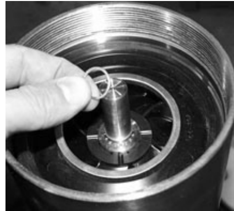
Figure 7-41 - Install Snap Ring, 8500-, 1250-Series
