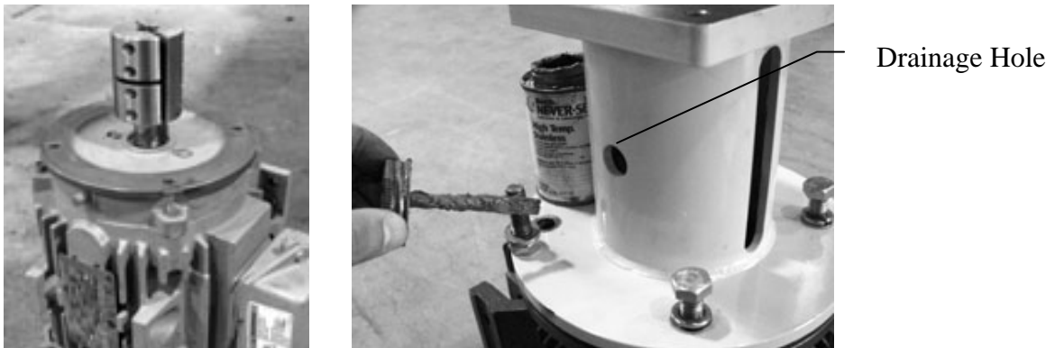
Figure 7-11 – Install Coupling and Bell Housing onto Motor
