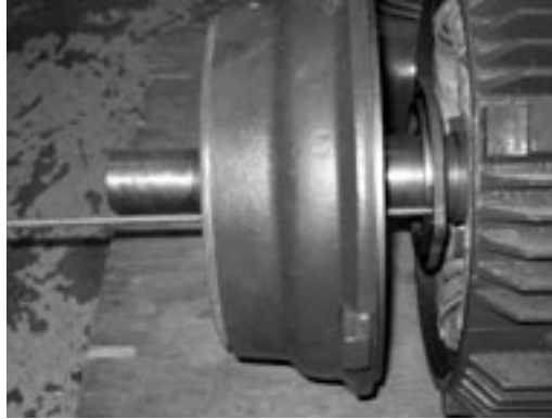
Figure 7-51 – Use All-thread to Align Retainer Plate
