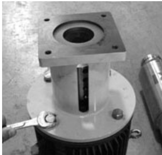
Figure 7-9 - Remove Bell Housing
