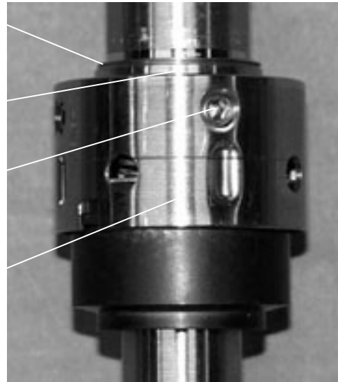
Figure 7-13 - Primary Seal Assembly
