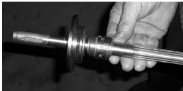
Figure 7-30 – Install seal and seal plate onto shaft
