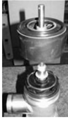
Figure 7-28 – Remove Shell and Stages
