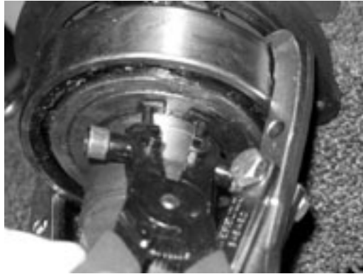
Figure 7-48 – Remove Bearing Retaining Ring
